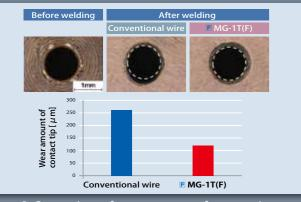
**Figure 2: Comparison of wear amounts of contact tips** Note: One hour continuous welding at 200A-25V, 100% CO<sub>2</sub> gas
