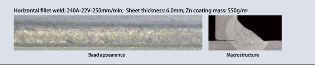
Figure 6: Bead appearance and cross-sectional macrostructure of E DW-1SZ (1.4mm dia.) weld
