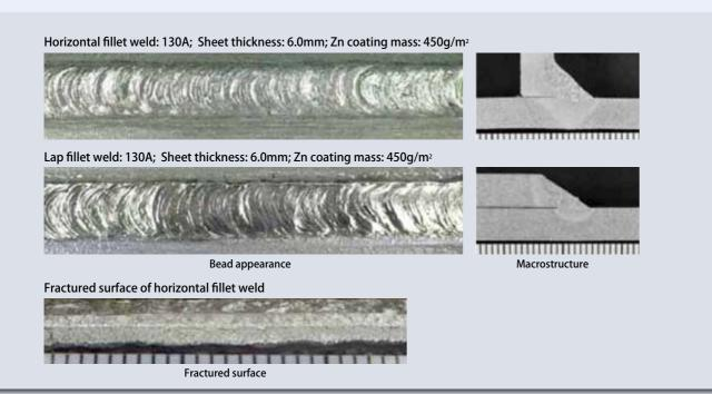
Figure 7: Bead appearance, cross-sectional macrostructure and fractured surface of E Z-1Z (4.0mm dia.) weld
