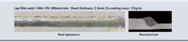
Figure 5: Bead appearance and cross-sectional macrostructure of E MX-100Z (1.2mm dia.) weld
