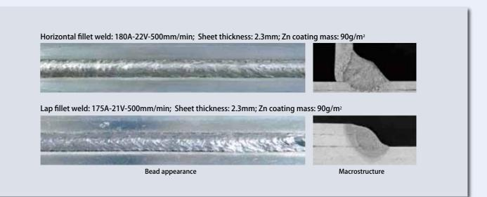
Figure 3: Bead appearance and cross-sectional macrostructure of E SE-1Z (1.2mm dia.) weld
