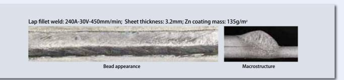
Figure 4: Bead appearance and cross-sectional macrostructure of E MX-1Z (1.2mm dia.) weld
