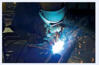
Figure 9: Welding a frame structure for a bus with E SE-1Z
