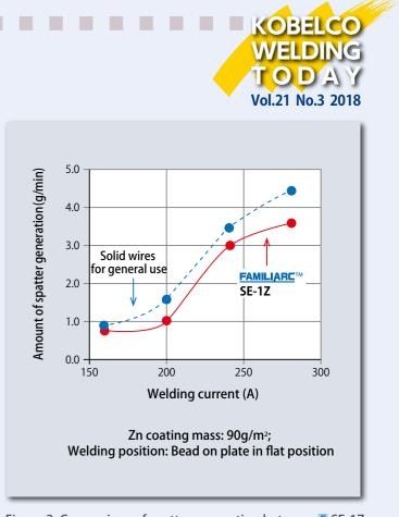
Figure 2: Comparison of spatter generation between E SE-1Z and solid wires for general use
