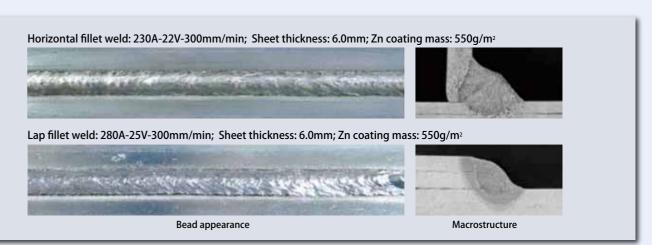
Figure 8: Bead appearance and cross-sectional macrostructure of E OW-1Z (1.2mm dia.) weld
