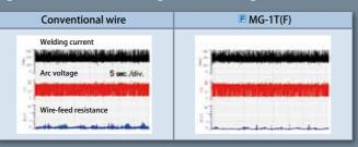
Figure 4: Time variation of welding current, arc voltage and wire feed resistance between a conventional wire and E MG-1T(F)
