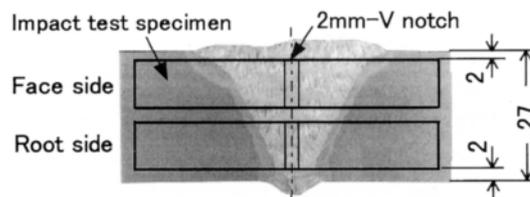
Fig. 2 — Location of impact test specimens removed from DW-55E welds (One-side welding with a ceramic backing material of FBB-3T)
