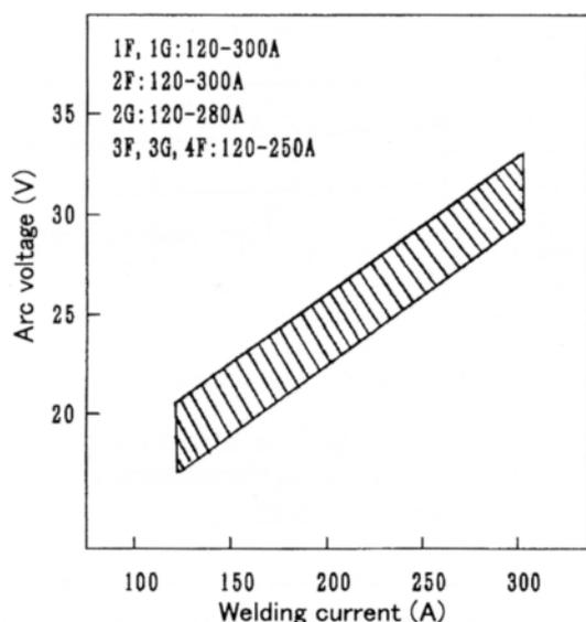
Fig. 3 — Proper ranges of welding currents and arc voltage (DW-55E, 1.2 mmØ); the welding positions of 2G, 3F, 3G and 4F restrict the use of high currents as shown in the figure respectively.
