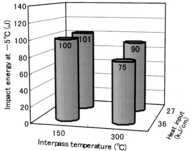
Fig. 5 — The effects of heat input and interpass temperature on Charpy impact energy (the average of 6 specimens) of MG-60 all-deposited metal
