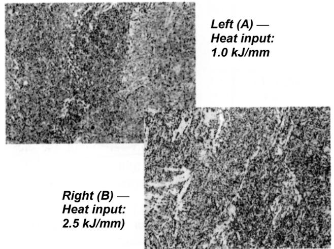
Fig. 2 — A comparison of microstructures of gas metal arc welded all-deposited metals of an ER80S-G trial wire, using two different amounts of heat input (X400) (Source: IIW Doc. XII-1647-00, 2000)
